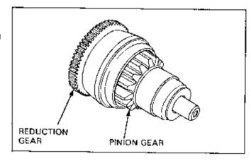
Check if the pinion gear moves smoothly along the axis.
