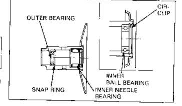
Drive a new outer bearing into place with the sealed end toward the outside.
