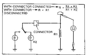
When the ohmmeter is connected in series, resistance values are large.
