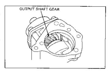
Contact is normal if Prussian Blue is transfered to the approximate center of each tooth and slightly to the side.
