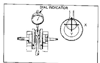
Measure the crankshaft runout using dial indicators.
