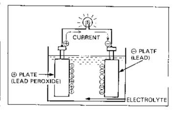
When you charge the lead/acid battery, electrolysis breaks the water down into its components, hydrogen and dxygen. Because of the generation of these gases, you must remove the filler plugs while charging the battery.
