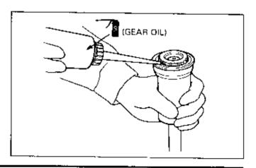
Hold the drive shaft upright to avoid spilling the damper case oil.
