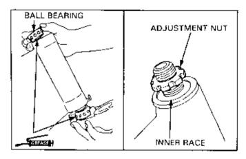
While holding the steering stem with one hand, install the top race and bearing adjustment nut onto the stem.
