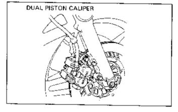
With the exception of in-board disc brakes and the GL1500 front brakes, all brake discs are exposed. To protect them from rust, the discs are made of stainless steel alloy.
