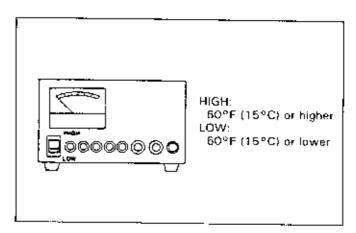
Push in the appropriate test button for three seconds and read the condition of the battery on the meter.
