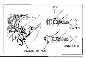
Minor adjustment is made at the lever end of the cable. It is necessary to turn back the lever dust boot to gain access to the adjuster.
