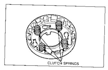
Assemble the drive plate in the clutch outer.
