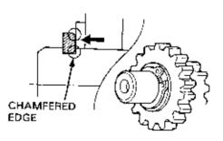
Grease or oil sliding or turning parts with the recommended lubricant before reassembly.
