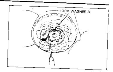
Hold the clutch outer using the clutch outer holder.
