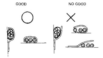
■ To unlock wire harness or hose from a clip, use a screwdriver to open up the tab. When locking the clip, press firmly until it clicks. If the clip was removed from the frame, replace it with new one.
