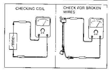
How to measure resistance using an ohmmeter.
