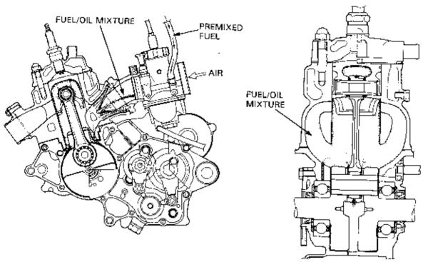
It is important to USE ONLY A 20:1 FUEL/OIL RATIO. All Honda engines are designed to operate most efficiently and with greatest durability using a 20:1 premix ratio. All standard carboretor jatting is based on this ratio.
