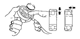
Ball bearings are always installed with the manufacturer's name and size code facing out. (Facing out meaning—thousand and sizing code should be visible from the side the bearing is installed from.) This is true for open, single-sealed and double-sealed bearings. Apply the proper grease to open and single sealed bearings before reassembly.
