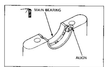
Mark a line perpendicular to the bearing surface from each edge of the notch as shown.
