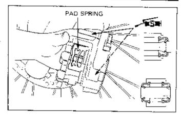
Install the new pad, align the holes in the pad and retainer and install the pad pin. Note the installation direction of the pad.
