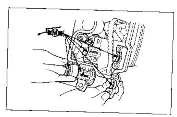
Fill the oil pockets in the head with the recommended oil.
