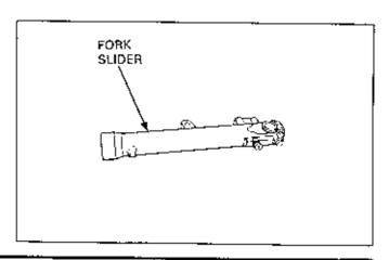
Check the fork piston and other components for damage, cracks, straightness or abnormal wear. Replace if necessary,
