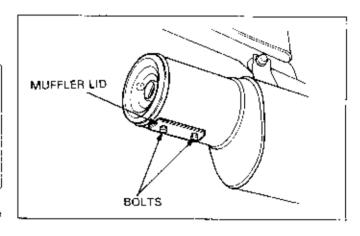
Start engine and rev it up to blow accumulated carbon deposits out of the muffler.
