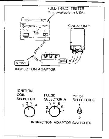
For digital-controlled spark unit, use spark adaptor (07508-0013600).
