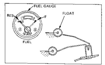
Measure the resistance between the connector terminals with the float in up and down positions.
