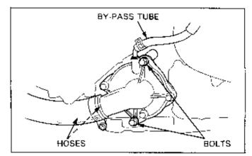
Remove the bolts and separate the pump cover from the body.
