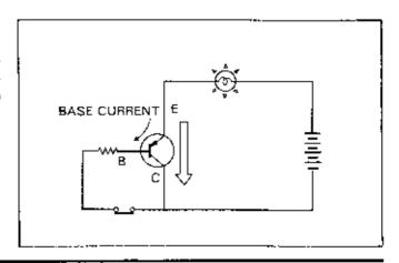
In the NPN type, almost no current flows when a positive voltage is applied to the collector and a negative voltage to the emitter. When a small current flows from the base to the emitter, a large current flows from the collector to the amitter.
