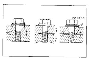
Certain areas of the motorcycle or scooter are subject to repeated and severe external forces. Special bolts with a high percentage of elastic deformation capability are used in these areas.
