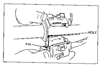
Apply a light coating of grease to the throttle cable ends and throttle grip sliding surface.
