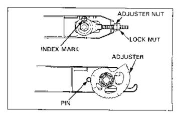
After adjustment, retighten the axis nut to the specified torque.
