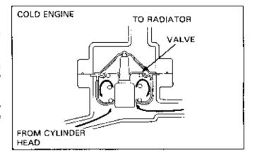
Even if atmospheric temperature varies, the thermostat controls the engine temperature at a constant level.
