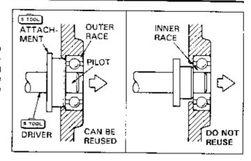
If the bearing is in a blind hole in the crankcase and cannot be removed by hammering on the apposite side, remove it with a bearing removers. For recommended bearing removers, refer to the Tool Compatibility Charts on page 1-15.
