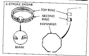
In 2-stroke engines, the piston has locating pins that hold the piston rings away from the intake and exhaust ports.
