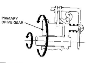
In some cases, a roller is used instead of a clutch weight between the drive plate and the clutch plate. In this type, centrifugal force shifts the roller to the outside of the drive plate, causing the pressure on the clutch plate to engage the clutch.
