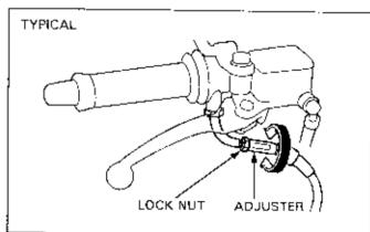
Major adjustments are made on the carburator and of the cable, with one of the adjuster types shown here.
