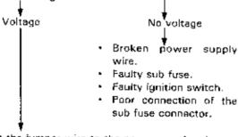
Connect the jumper wire to the power supply wire and oil level indicator wire to short and check for voltage between the indicator wire and ground.
