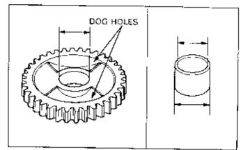
Calculate the gear-to-bushing clearance; replace the component if the service limit is exceeded.
