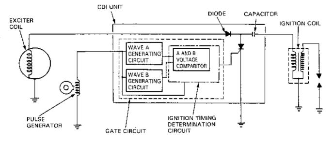
The pulse generator produces positive and negative voltage pulses when the rotor reluctor crosses the generator.
