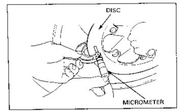
Check the brake disc for warpage.
