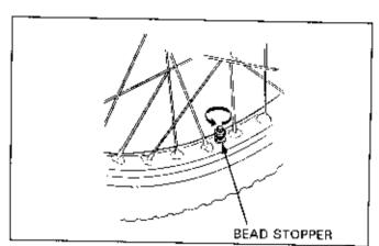
Collapse in the bead with a tire bead breaker.
