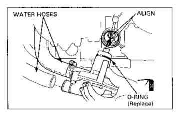
Tighten the pump mounting bolts.
