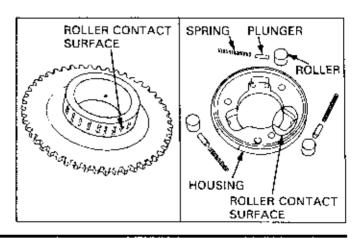
For one-way sprag clutch, check each sprag, clutch housing, and all inner portion contact surfaces.
