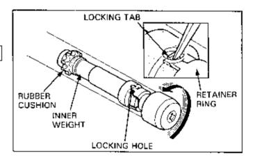
Install a new retainer ring to the inner weight and install the end weight, aligning the cutout.
