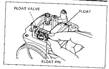
Check the float valve and valve seat for scores, scratches, clogging and damage. Replace if necessary.
