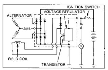
Date of Issue: Sep., 1985 © HONDA MOTOR CO., LTD. The voltage regulation is performed by a high frequency ON/OFF cycle of the alternator. When the DC voltage of the output waveform is measured by a voltmater, a value smaller than the peak voltage is measured.
