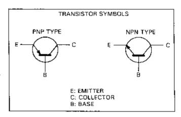
In PNP type transistors, when a positive voltage is applied to the emitter and negative voltage to the collector, almost no current flows from the collector to the emitter. If the emitter voltage is raised slightly higher than the base voltage and a small amount of current flows from the emitter to the base, a large amount of current flows from the emitter to the collector.
