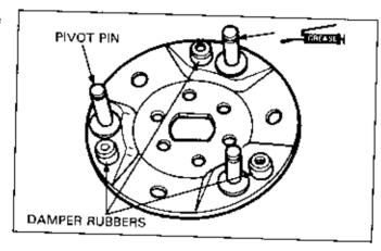
Install new clutch shoes on the pivot pins and push them into place.
