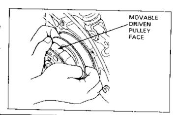
Remove the pulley assembly once with the drive belt installed.
