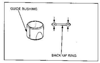
Check the fork sliders for internal scretches, dents that are visible from both the inside and outside, or abnormal wear. Replace if necessary.
