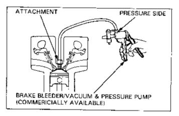
Squirting a little scapy water around the cylinder and head mating area will tell you if the head gasket is leaking to the outside atmosphere. Checking for bubbles in the cooling system of a liquid-cooled machine will tell you whether or not the head gasket is leaking into the cooling passages. The only thing this test won't tell you is the difference between a head gasket leak into the adjacent carn chain (or gear) well, and a leak past the piston rings.
