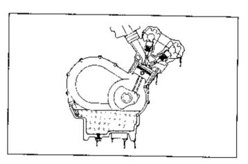
Remove either the oil level gauge or filler cap to allow rapid draining.
