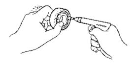
Ball bearings are checked (after cleaning) by slowly rotating the inner race while holding the outer race stationary. If any radial play or roughness is falt, it must be replaced. The bearing should have no axial play; if it has noticeable axial play, it must be replaced.
