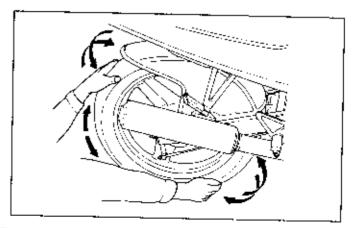
Check for looseness of bolts/nuts in connection with the following.
