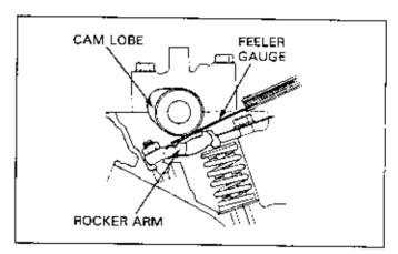
In the case of valve lifters in direct push-type engines, the clearance between the cam lobe and lifter or shim is measured with a feeler gauge.
