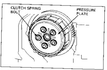
Remove the lifter rod, push rod, discs and clutch plates.
