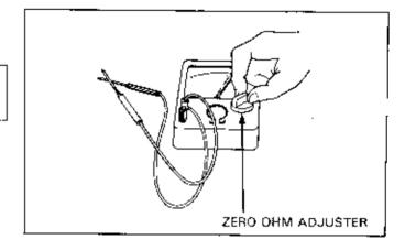
Since the polarity of terminals is not important, either probe may be applied to the terminal. However, since diodes allow current to flow in one direction only, the polarity is important.
