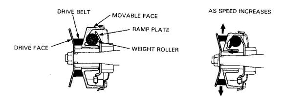
As the engine rpm increases, centrifugal force on the weight rollers is increased. This pushes the movable drive face toward the fixed face. This reduces the drive ratio by allowing the drive belt to run on a pulley of greater diameter.
