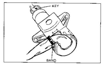
Push the contact base tabs in with a screwdriver so that they are out of the slots in the ignition switch body, and remove the contact base.
