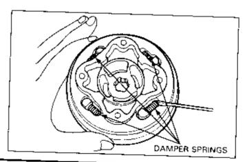
Install the primary drive gear onto the clutch assembly and compress the clutch springs using the clutch spring compressor, then remove the set ring.
