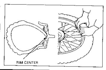
Apply a mild detergent solution to the rim and tire mating surfaces.
