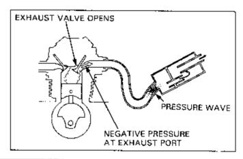
On 2-stroke engines, there is the possibility that the air/fuel mixture that was scavenged just before the end of the exhaust stroke may leak out to some degree and be discharged into the exhaust port.
