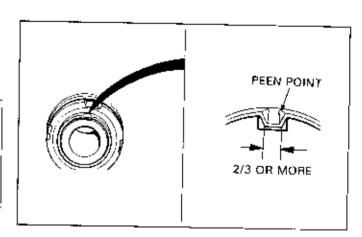
Set the bearing in the lifter plate, then install the clutch springs and the lifter plate.
