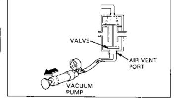
Connect the vacuum pump to the hose that goes to the vacuum tube fitting.
