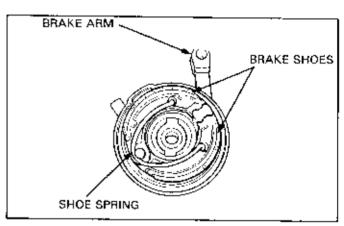
install the brake panel on the wheel hub.
