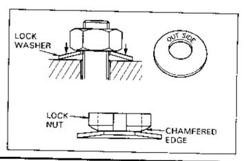
Tighten the lock nut to specified tarques using a special tool.
