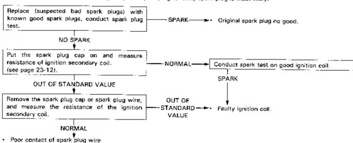
Faulty spark plug wire or faulty spark plug cap
