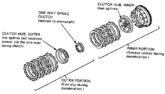
The major difference between this system and a conventional clutch is a two-piece clutch hub, inner and outer. In addition, the outer portion of the clutch hub, that which controls the majority of the clutch plates and discs, is driven by a special one-way sprag clutch.
