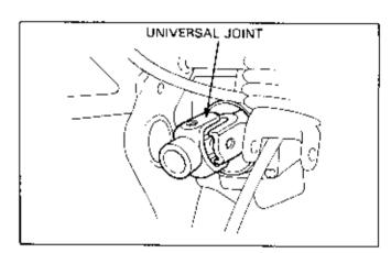
Check that the universal joint moves smoothly without binding or noise.
