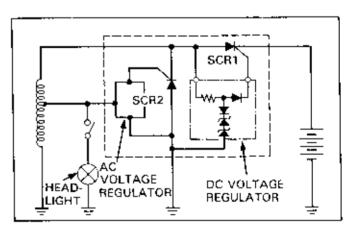
The output of the alternator goes to the gate of SCR1 via the DC voltage regulator. When the voltage at the cathode of the SCR1 is less than the voltage at the gate, it is turned ON and thus SCR1 conducts current to the battery. When AC output of the alternator changes from the positive to negative, the gate voltage of SCR1 becomes zero, hence turning OFF the SCR1 and cutting off the negative signal to the battery.
