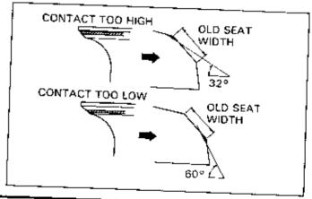
Using a 45 degree cutter, remove any roughness or irregularities from the seat.
