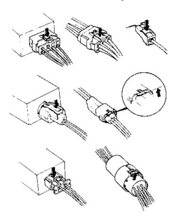
When separating connectors, pull only on the connector indusing. Do not pull on the wires.
