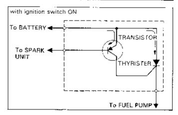
While the engine is running, pulses are transmitted from the spark unit to the ignition primary circuit and, when it is transmitted to the transistor, current flows from the transistor to the thyrister to turn it ON. The battery current flows to the fuel pump this way.
