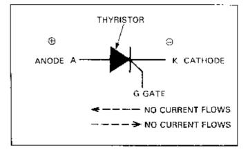
The thyristor is turned on when a certain amount of voltage is applied to the gate. This input to the gate is called gate voltage or trigger voltage.
