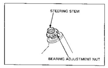
Move the steering stem right and left, lock-to-lock, several times to seat the bearings.
