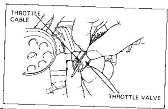
Remove the jet needle retainer and jet needle from the throttle valve.
