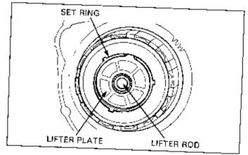
Shift the transmission into top gear and apply the rear brake. Remove the lock nut.
