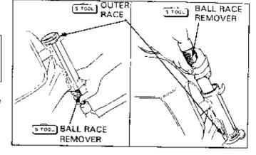
Install new races into the steering head of the frame using the driver and attachment.
