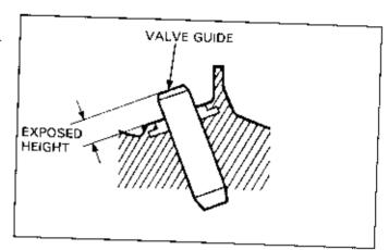
Chill the valve guides in the freezer section of a refrigerator for about an hour.
