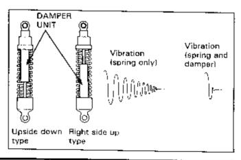
In addition to the inverted and conventional damper body types, there are two basic damper designs, each named for the method used to create the damping action; the friction type and the oil damper type.
