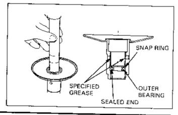
Install in a new inner bearing.
