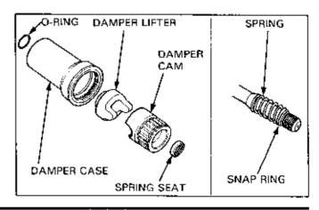
Date of Issue: Sep., 1988 © HONDA MOTOR CO., LTD. Remove the oil seal, oil seal guide and damper spring from the damper case.
