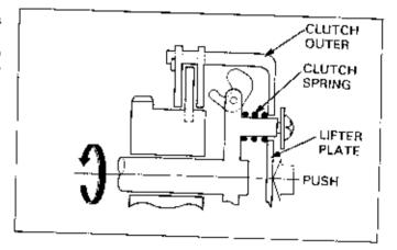
As the pedal is released after completion of shifting gears, the lifter cam returns to its original position. When the clutch outer returns to its original position by the tension of the clutch spring, the disc and the plate closely join again, and the clutch is then engaged.
