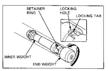
Insert the weight into the handlebar and align the spring pinholes by turning it.
