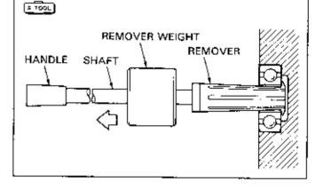
If the use of a bearing remover is not possible, remove the bearing by thermally expanding the case; slowly and uniformly heating the case with a heat gun (industrial dryer).
