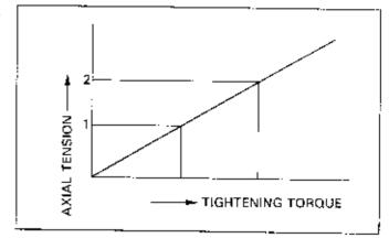
It must be noted that, in this control method using torque values, the axial tension is proportional to the torque under certain conditions. Under other conditions, this important axial tension varies even when the fastener is tightened to the same torque.
