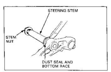
Date of Issue: Sep., 1988 © HONDA MOTOR CO., LTD. Install a new dust seal and bottom race onto the steering stem,
