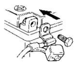
After completing the job, check that all terminal protectors are placed correctly.
