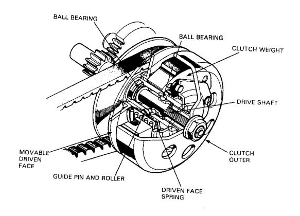
The centrifugal clutch is disengaged when the engine speed is low. When engine speed increases, the rotating clutch shoes of the clutch weight will expand as the centrifugal force increases. In this way, the clutch is automatically engaged.
