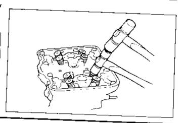
Clean any gasket material from the cyfinder mating surface. Reface the mating surface using oil stone, if necessary.
