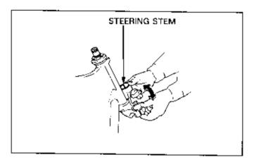
Retighten the bearing adjustment nut to 15 N·m (1.5 kg-m, 10 ft-lb), then loosen the adjustment nut 1/8 turn.
