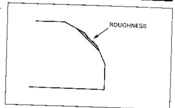
Using a 32 degree cutter, remove 1/4 of the axisting valve seat material.
