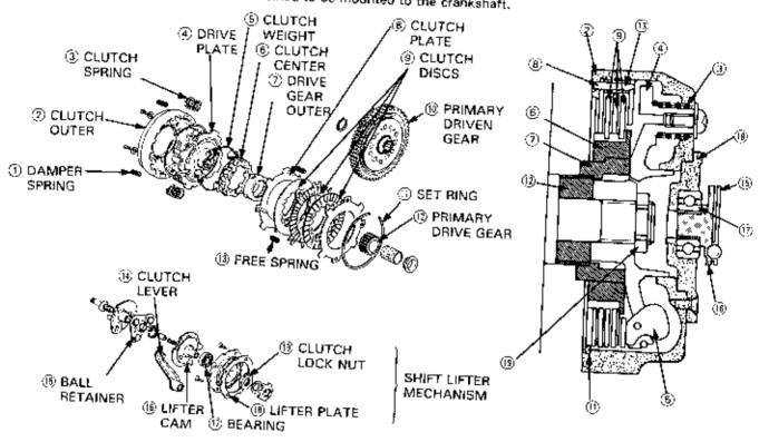
At low engine speeds, the centrifugal force applied on the clutch weight is less. The weight does not work, and a gap exists between the clutch plates and discs. The clutch is disengaged.
