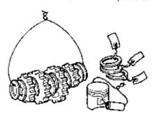
Reassambly position of critical parts should be noted before the parts are disassembled. This will allow those dimensions (depth, distance, or position) to be correctly duplicated upon reassembly.
