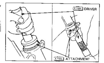
On aluminum frames: replace the races using the Ball Race Remover Set as described in the following procedure.
