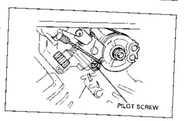
Turn the No. 1 carburetor pilot screw counterclockwise to the final opening from the position obtained in step 8.
