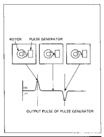
The output from the pulse generator is converted into basic waves A and B.
