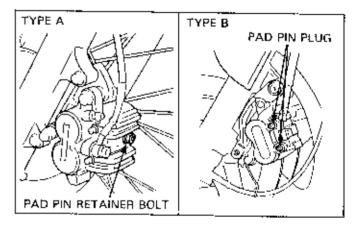
Apply the brake lever to force the caliper piston out of the caliper.
