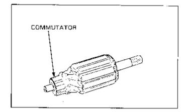
Check for continuity between pairs of commutator bars.
