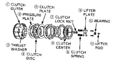
When the clutch lever is pulled in, the clutch lifter mechanism presses the pressure plate through the lifter plate, resulting in a gap between the disc and the plate. The power of the crankshaft is now not transferred to the rear wheel.
