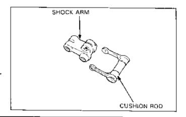
Check the pivot collars, dust seals, bushings and/or bearings for wear or damage and replace if necessary.
