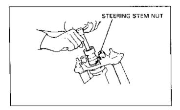
The lack washer tab must be bent down in order to remove the lock nut.
