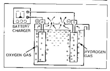
Because the motorcycle battery is constantly subjected to charging and discharging cycles, the water in the electrolyte is boiled off.
