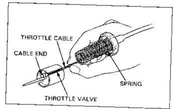
Align the cutout in the throttle valve with the throttle stop screw on the carburetor body and install the valve on the carburetor.
