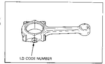
Record the corresponding crankpin O.D. code letter (A, B or C) or measure the crankpin O.D.
