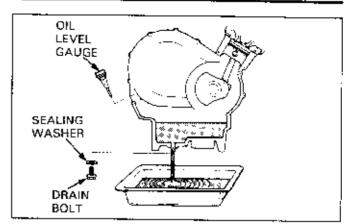
Pour the recommended engine oil into the engine through the oil level gauge/filler hole. The oil filler hole and cap are separated from the oil level gauge on some engines.
