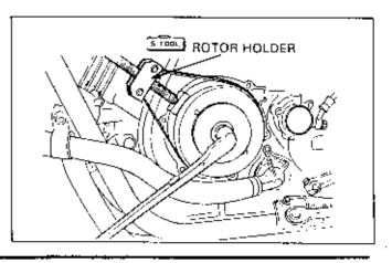
Insert flywheel puller into the rotor and remove the rotor.
