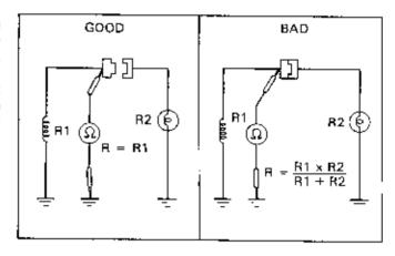
Similarly, if a circuit has branches, the connector leading to the specific branch needs to be disconnected in order to read correctly.
