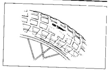
Tread depth can be observed directly or by use of the depth gauge,
