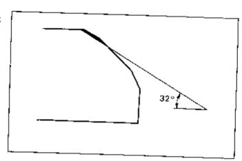
Using a 60 degree cutter, remove the bottom 1/4 of the old seat,
