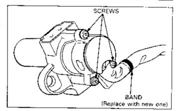
When the contact base is secured with tabs; Remove the ignition switch and band.
