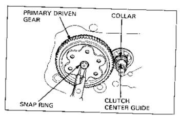
install the clutch assembly onto the crankshaft,
