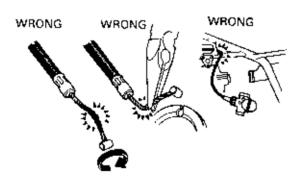
Rubber parts can deteriorate with age and are highlysusceptible to damage from solvents and oils. Check these parts before reassembly and replace as necessary. Loosening a part with multiple fasteners sizes should be done from the outside-to-inside in a crisscross pattern, loosening the small fasteners first. Loosening the big fasteners first will place an excessive force on the smaller fasteners.
