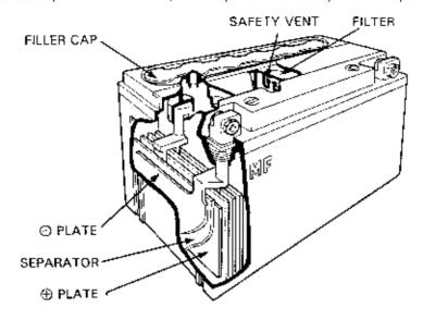
Similar in design to the conventional battery, the MF battery produces hydrogen and oxygen gas. However, the plates are designed not to convert to lead completely. (This state of lead is called sponge lead.)
