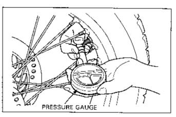
Check for cracks and damage to the tire tread and walls and replace the tire if necessary.
