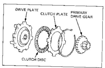
Compress the clutch springs with the clutch spring compressor, then install the set spring in the groove of the clutch outer.
