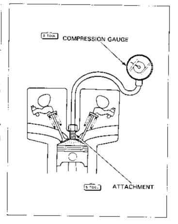
If compression is low, drop small amount of clean engine oil into the cylinder, then recheck the compression.
