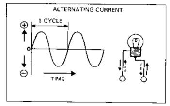
In motorcycles, all electricity generated is AC. However, AC can be converted to direct current (DC) by rectification. The DC current is then supplied to components operating on DC. For example, some models use DC for their headlights and others use AC.
