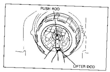
Install the bearing in the lifter plate, then install the clutch springs, pressure plate, washer(s) and clutch spring bolts.
