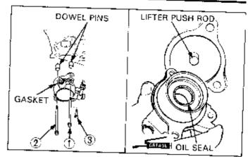
Tighten the mounting bolts to the specified torque.
