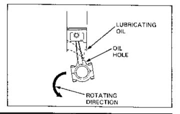
Date of Issue: Sep., 1988 © HONDA MOTOR CO., LTD. Install the bearing caps and connecting rods on the correct crankpins,
