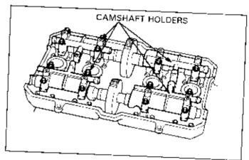
Remove the camshaft holders and measure the width of each plastigauge. The widest thickness determines the oil clearance.
