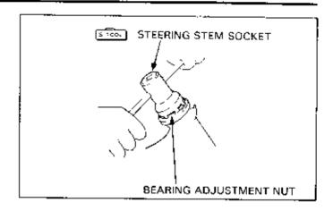
If the bearings are the loose-ball type, place a shop towel under the steering stem to catch the steel balls,
