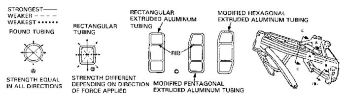
The frame also serves to absorb vibration from the engine and, to some degree, from the road surface. The difference in basic frame structure is determined according to the engine type and the type of use the machine is designed for.
