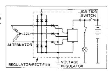
The rectified waveform of the triple phase AC output is more stable than the single phase AC type.
