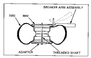
With the breaker arm in the horizontal position, place the breaker press head assembly over the breaker arm press block. Make sure the press head bolt is backed out all the way and then position the nylon buttons on the press head against the inside edge of the rim.
