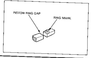
The oil ring is needed to remove oil from the cylinder wall and return the residue from the hole of the oil ring groove. If the oil ring fails, oil flows into the combustion chamber and burns, causing smoke. The oil ring is either of a split type arranged with two side rails and a slotted expander, or an integral type with a slotted square edge.
