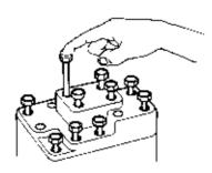
Torquing multiple sized fasteners should be done as follows: tighten all to hand-tight, then torque big fasteners before little fasteners. Torque pattern should be crisscross from inner-to-outer. To minimize distortion, critical fasteners should be torqued in two or three increments. Unless specified otherwise, bolts and fasteners are installed clean and dry; do not use oil on the threads.
