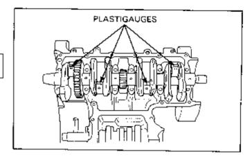
Install the bearing caps and rods on the correct crankpins, and tighten them evenly.
