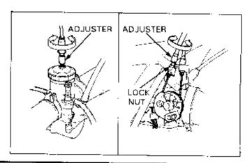
If the throttle cable has an adjuster anywhere within its length besides the ends, major adjustment is made there.
