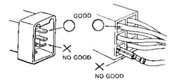
Check for tern protective covers and oversized, loose fitting, female terminals before installation.
