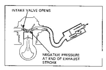
The discharged gas flows through the muffler forming a high speed pressure wave. Due to the inertia of liquid mass, negative pressure is applied to the exhaust port where the pressure wave had passed. When the exhaust valve (or port) opens on the next exhaust stroke, the exhaust gas is drawn out by the negative pressure, and the exhaust efficiency is improved.
