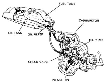
The amount of lubricant delivered to the engine is dependant on both engine rpm and throttle position.
