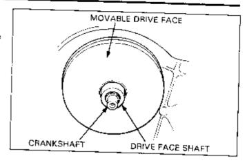
Remove the three bolts attaching the movable drive face seal and remove the seal.
