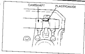
Install the camshaft holders and tighten the mounting bolts to the specified torque. (Refer to the Model Specific manual for the correct torque specification)
