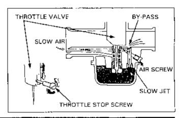
Piston valve type throttle valves have a cut-out on the intake side. The larger the cut-out, the greater the volume of air entering and the leaner the mixture.
