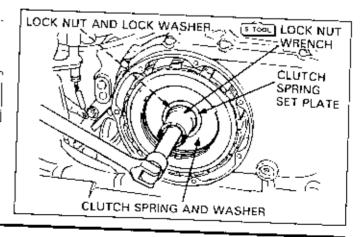
Remove the clutch pressure plate, clutch plates and discs.
