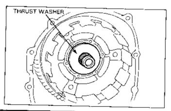
Coat the clutch discs and plates with clean oil,
