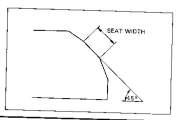
After cutting the seat, apply lapping compound to the valve face, and lap the valve using light pressure.
