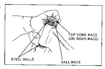
Remove the dust seal and top cone race, or inner race, while holding the steering stem with your other hand. Then remove the steering stem from the frame.
