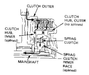
When there is a backloading on the clutch caused by the rear wheel nearing lock up, the sprag clutch will slip just enough to prevent the wheel from locking without losing the benefit of maximum engine compression braking.
