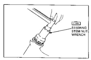
Reinstall the top bridge and fork legs temporarily.
