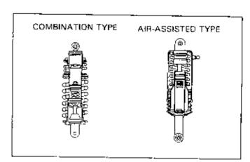
The right "shock" on GL1500s is actually only an "air spring". It has no dampening properties aside from a very slight seal friction and is filled with only a very small amount of oil to lubricate its shaft and oil seal.
