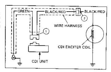
If, while measuring resistance at ①, the negative probe is placed on the ground wire (green), then the connection to ground is checked as well.
