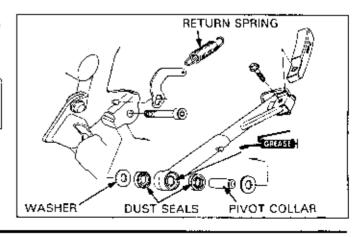
Inspection For Side Stand With Ignition Cut-off Switch
