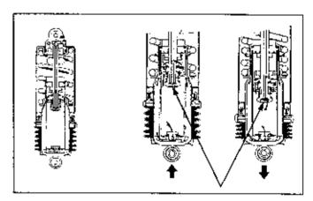
Decreasing the orifice diameter increases resistance and damper hardness.
