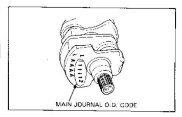
Cross reference the case and journal codes to determine the replacement bearing color code.
