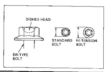
UBS bolts are in the high-tension category. They can be recognized by undercuts under their bolt necks. UBS bolts are marked either with or without strength marks. Furthermore, these bolts are so structured so they will not easily loosen, by the provision of a slight slope of 5 to 60° on the bottom of the flange.
