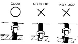
■ Do not squeeze a wire against a weld or the end of its clamps.
