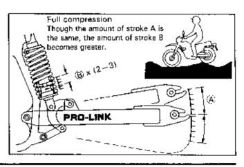
This arrangement offers a greater amount of suspension stroke compared to the amount the damper unit compresses and therefore greater control for improved suspension performance. It also enables the weight of the spring/damper unit to be centralized more compactly, nearer the center of the frame.
