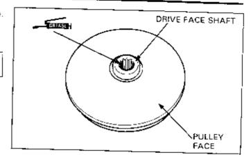
Install the movable face assembly on the crankshaft.
