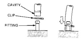
Rubber or Plastic Dust/Dirt Boots should be replaced securely in the exact positions they were designed for.
