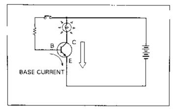
Transistors also resemble switching devices. The transistor is turned on, allowing collector to emitter current to flow when there is base current, and turn off when no base current exists.
