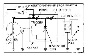
The capacitor cannot discharge until the SCR is turned ON. The SCR is turned ON as the pulse generator sends pulses to the trigger circuit which, in turn, feeds current to the gate of SCR.
