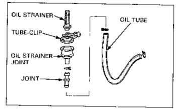
Clean strainer screen by blowing it out with compressed air. To replace screen, reverse the removal procedure.
