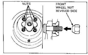
Install the wheel in its original position.
