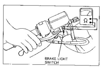
2. If normal, disconnect the brake light switch connector and check for continuity between the terminals while operating the brake lever (or padal).
