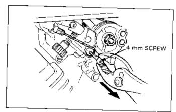
Turn the screw in and carefully count the number of turns until it seats lightly. Make a note of this to use as a reference when reinstalling the screw.
