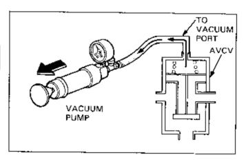
Connect the vacuum pump to the air vent fitting on the AVCV that goes to open eir.
