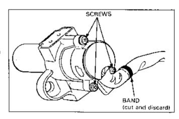
Reassemble the switch and cylinder with the cylinder shaft aligned with the hole in the switch.
