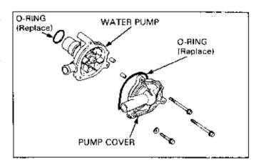
Install a new O-ring onto the water pump.
