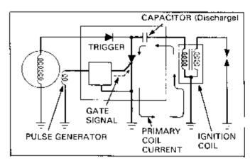
When the SCR is turned ON, the capacitor discharges current to the ignition primary coil. A high voltage surge included in the secondary coil jumps the spark plug gap.
