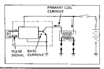
As the engine speed increases, the duration of current flow through the primary coil becomes shorter and thus the secondary coil voltage does not go high enough. For this reason, the ignition timing control circuit controls the duration of current flow through the ignition primary coil.
