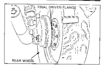
Set the rear wheel in place and install the axle. For mechanical drum brakes, connect the brake rod (or cable) to the brake arm and install the adjusting nut loosely. Connect the torque rod to the brake panel and tighten the torque rod nut to the specified torque.
