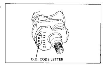
Cross-reference the crankpin and rod codes to determine the replacement bearing color.
