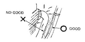
Protect wires and harnesses with at least two layers of electrical tape or with electrical harness tubes if they contact a sharp edge or corner,
