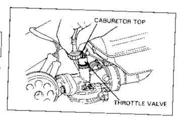
While compressing the spring, disconnect the throttle cable from the throttle valve.
