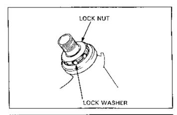
Remove the bearing adjustment out.
