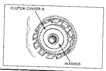
Install the clutch center 8, the one-way clutch and one-way clutch inner as an assembly onto the clutch outer.
