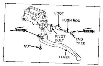
Place the master cylinder on the handlebar and install the holder with the "UP" mark facing up.
