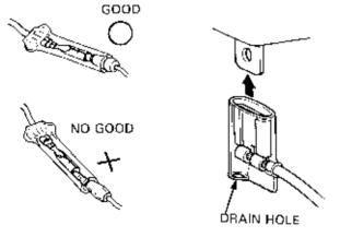
Secure wires and wire harnesses to the frame with wire bands at the designated locations. Install the bands so that only the insulated surfaces contact the wires or wire harnesses.
