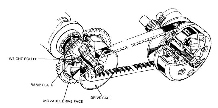
The drive pulley consists of a fixed and a movable face. The movable face is capable of sliding axially on the shaft of the fixed face. The ramp plate, which pushes the weight rollers against the drive face, is attached to the shaft of the drive face with a nut.
