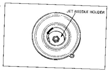
Check the jet needle for stapped wear and replace if necessary.
