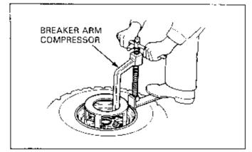
Screw in the breaker arm compressor bolt while pushing the breaker arm on the tire with your foot to break the bead from the rim.
