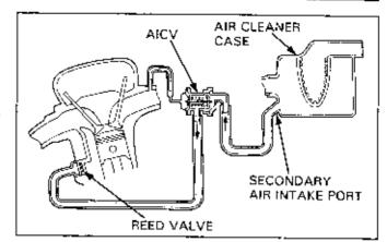
Disconnect the air cleaner-to-air injection control valve hose from the air cleaner case.
