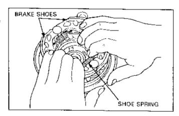
Remove the following from the brake panel.
