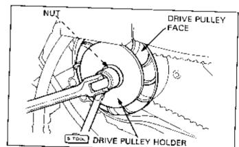
If the drive pulley holder cannot be used, remove the cooling fan at the right side of the crankshaft, and hold the flywheel with the universal holder.
