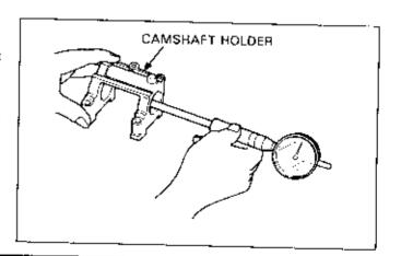
If a dial indicator cannot be used, measure the oil clearances using plastigauge:
