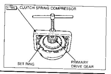
Install the clutch damper springs.
