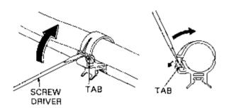
Check that the wire harness does not interfere with any moving or sliding parts after clamping.
