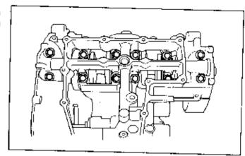
Remove the lower crankcase and measure the compressed plastigauge on each journal.
