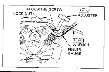
When the lock nut is tightened, the clearance may change. So be sure to recheck the clearance after tightening the locknut.
