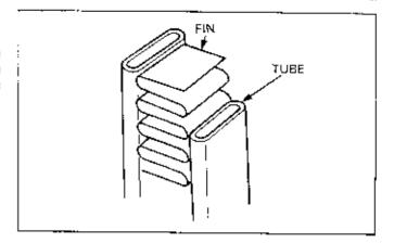
It is important that air is permitted to pass through the radiator fins so that the heat is dissipated from the coolant to the fins and into the atmosphere. Crushed or twisted fins will not permit heat to be dissipated because of inability of the air to pass through them, resulting in lowered cooling capacity. If 1/3 or more of the fins are crushed or twisted, the fins should be repaired using a small flat blade screwdriver.
