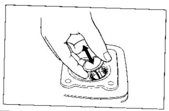
Measure and record the valve stem O.D. in three places along the valve guide stiding area.
