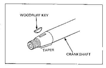
Set the rotor groove to the woodruff key and install the rotor on the crankshaft.
