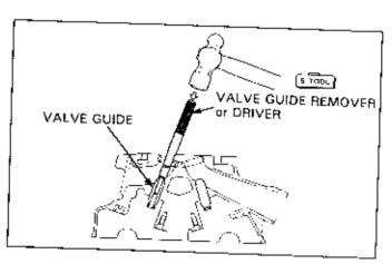
While the cylinder head is still heated, drive a new valve guide in from valve spring side until the exposed height is the same as was measured for the old guide.
