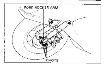
Check for oil leakage around the shock absorber piston rod. Inspect the rod for scoring, wear and peeling of the chrome plating on the working surface.
