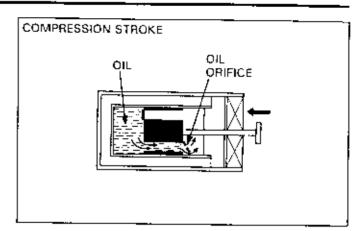
On the compression stroke, oil is forced through several large capacity damping orifices so that the wheel can respond quickly to terrain changes. Since the wheel is free to move quickly, the average ride height of the machine is not disturbed.
