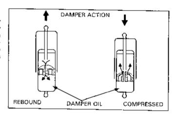
Oil dampers units are either the upside down type or the right side up type. Running the damper body upside down (with the shaft below and the body above) reduces unsprung weight.
