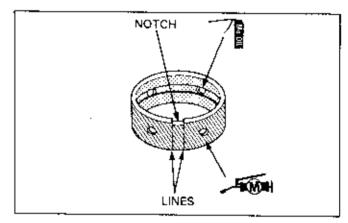
Place the bearing in the crankcase by aligning the two lines with the crankcase groove. Press it into place using a hydraulic press.
